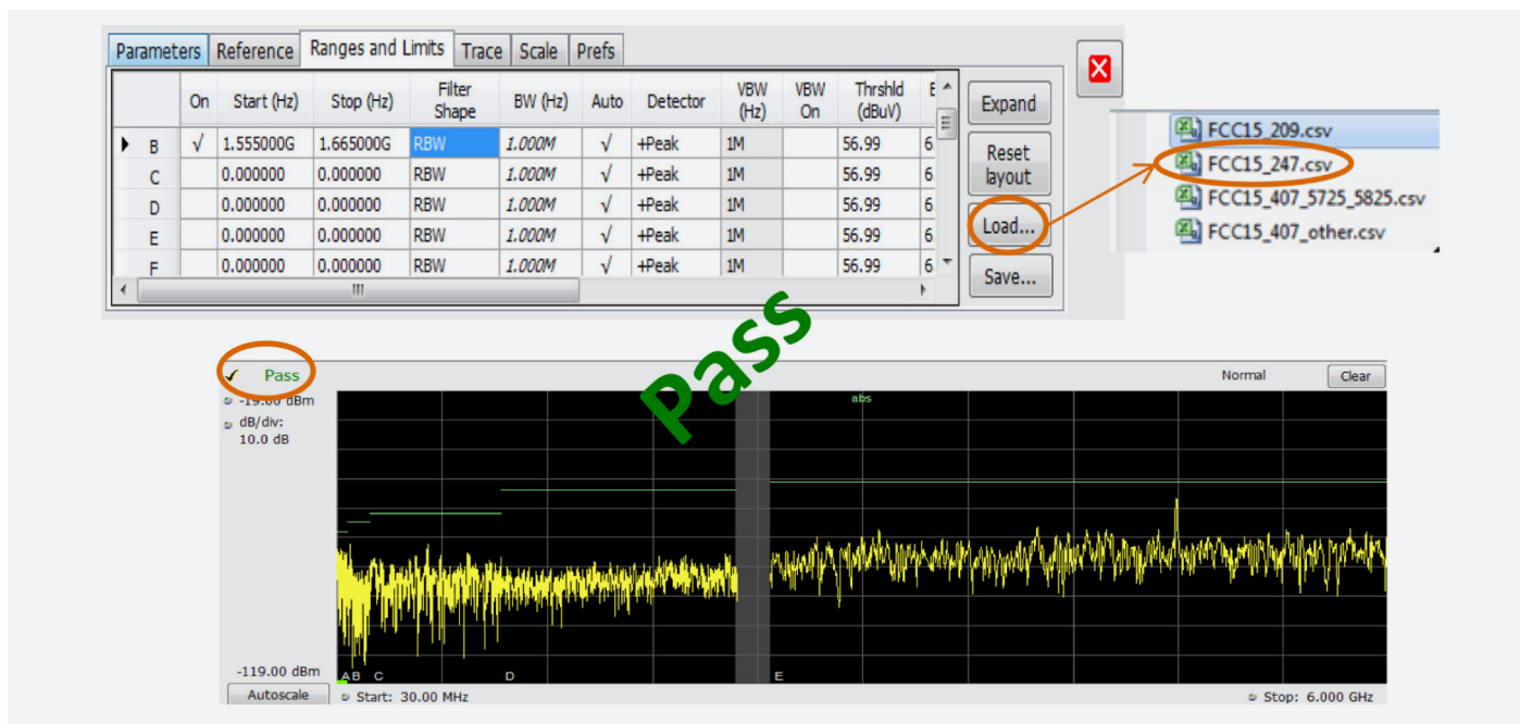
FIGURE 17. Example of Spurious Emission Test in FCC 15.247 signal (high deviation).
